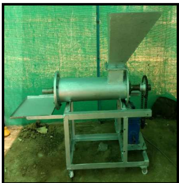
Fig. 3. Front view of fabricated pelleting machine
