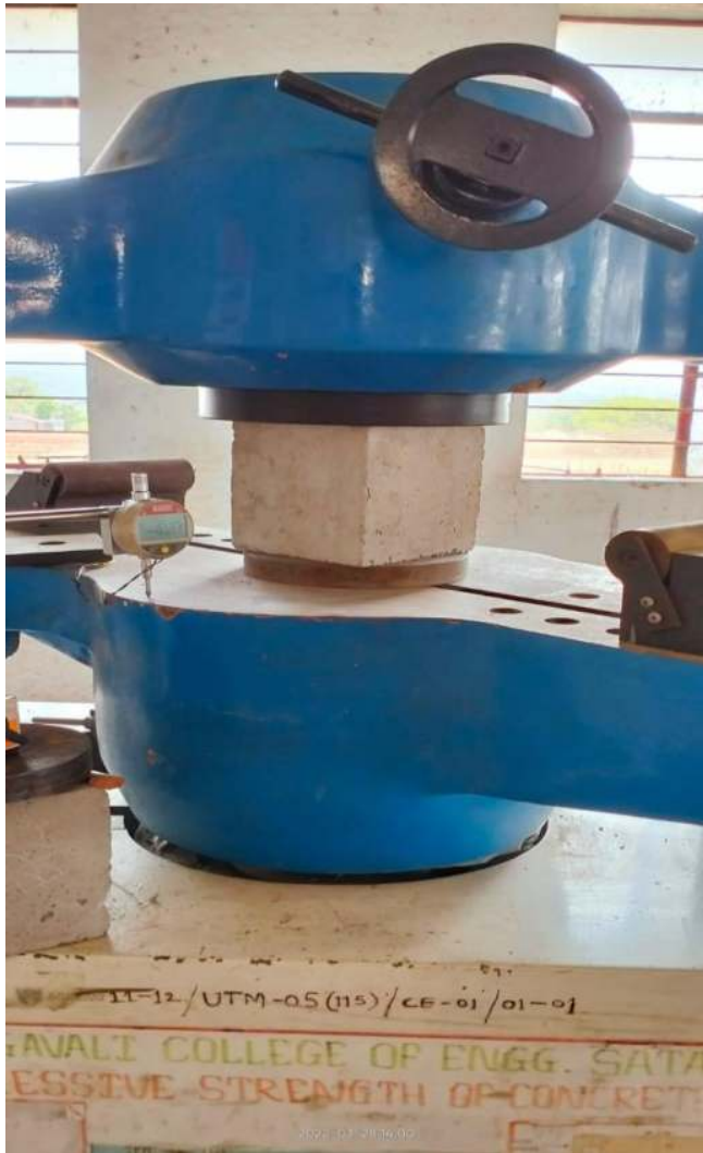
Cube Testing On UTM
