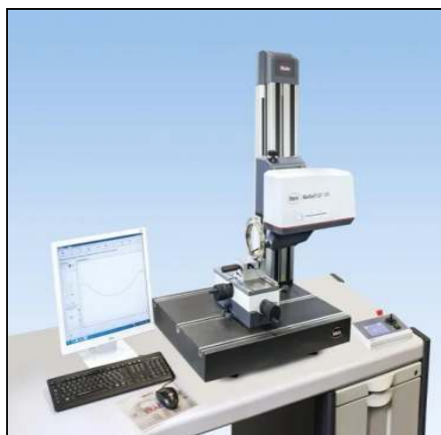
Fig.11. MarSurf LD 130 Combined Contour and Roughness Measuring Station[2], [69]
