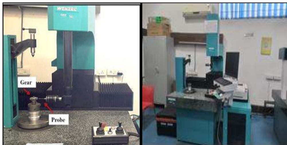
Fig.10. Wenzel GearTec Smart Gear 500 computer numerical control gear metrology [2].
